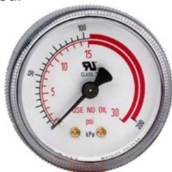
A change in the pressure gauge readings results in a failed drop test. A failed drop test confirms a leak exists, not the leak's location. Leak testing is required following a failed drop test. Leak testing uses a liquid solution, or another accepted method, to pinpoint the leak's location. Solutions must be compatible with the gas being checked. Never use a solution containing petroleum to check for an oxygen leak. Always test for leaks before transporting cylinders.
