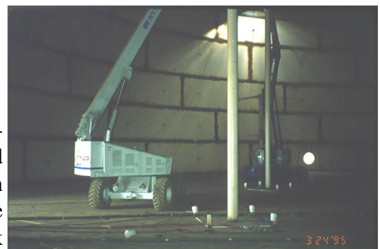
Propane-powered manlift in a large tank
