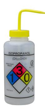
It is recommended you use a wash bottle with safety venting, which is indicated by the droplet with a slash-through-it symbol. Safety Venting prevents dripping.
